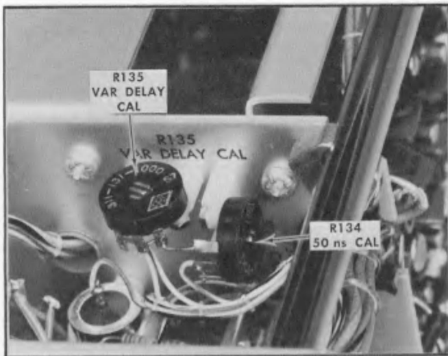
Fig. 5-21. Location of delay timing adjustments on the left side of the Type 115 chassis subpanel.
